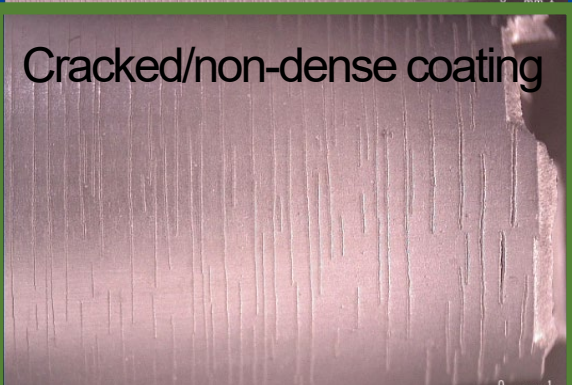
Cracked/dense coating
