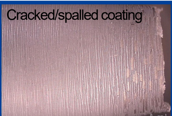
Cracked/non-dense coating
